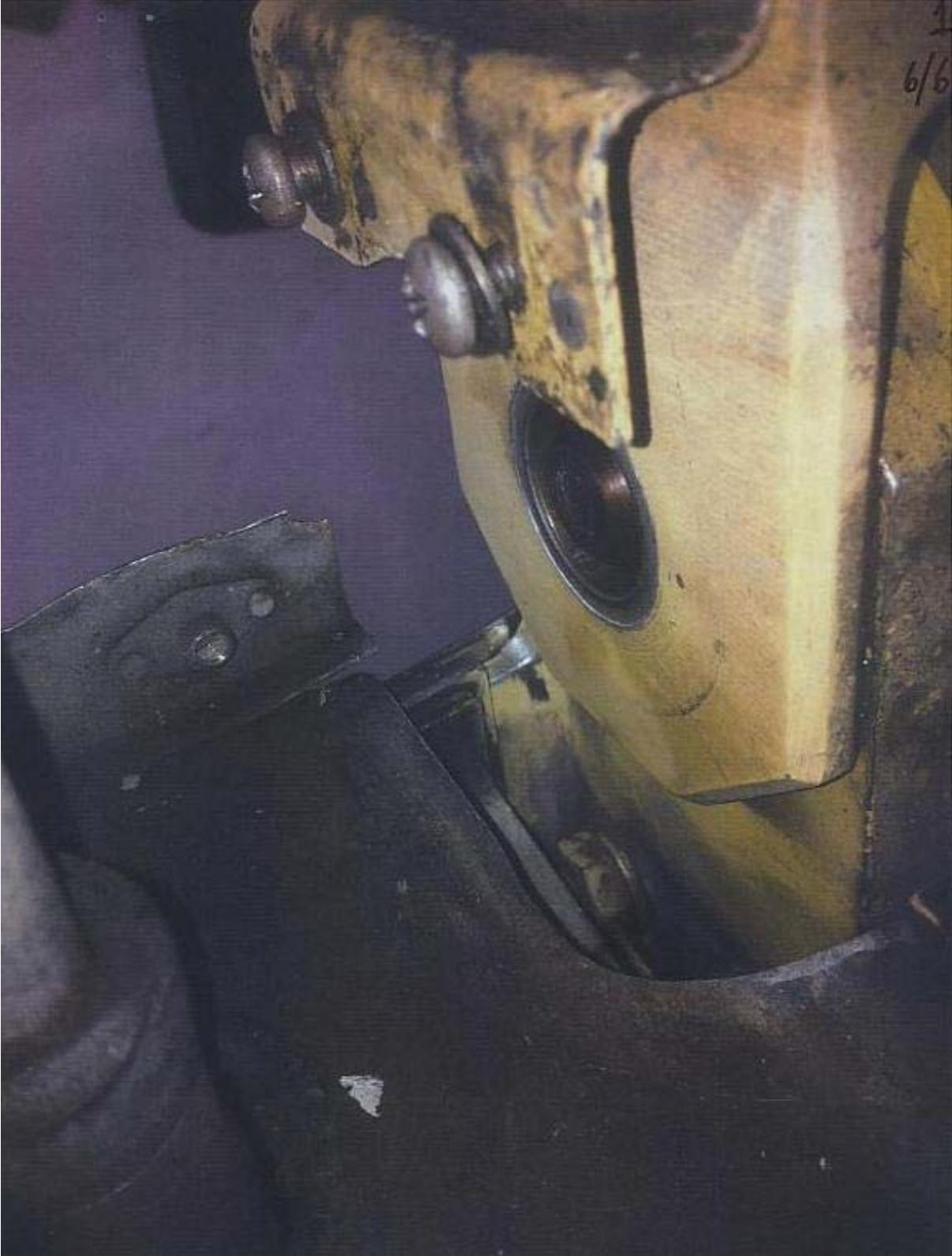
**Beechcraft B200, Cracked Spar Attach Fitting, ATA 5740**
